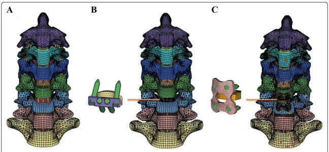
Fig. 1 A three-dimensional finite element model of a healthy C2–T1 segment (a) and two fusion models with 4-screw Zero-P (b) and the standard PCC (c) at the C5–C6 segment
