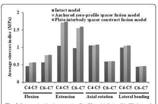
**Fig. 5** Stresses inside the superior C4–C5 and inferior C6–C7 discs of the intact model, the Zero-P fusion model, and the standard PCC fusion model
