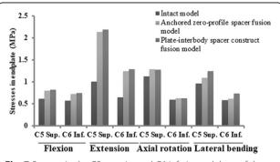
**Fig. 7** Stresses in the C5 superior and C6 inferior endplates of the intact model, the Zero-P fusion model, and the standard PCC fusion model
