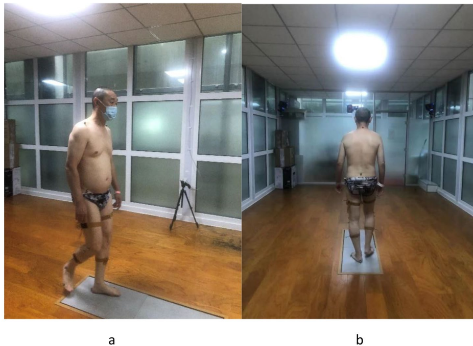
Fig. 4 Placement of 22 fluorescence tracking points according to the requirements of the DAVIS HEEL template. The patients underwent the 3D gait quantitative analysis system. According to the fluorescent marker placement standard of the DAVIS HEEL template, a fluorescent marker point was pasted on the subject. Fluorescent markers fixed on the calf and thigh with elastic bandages were placed on the outside of the patient's lower limbs as tracking points, with a total of 22 points. Figs a and b illustrate the patient's position during the test
