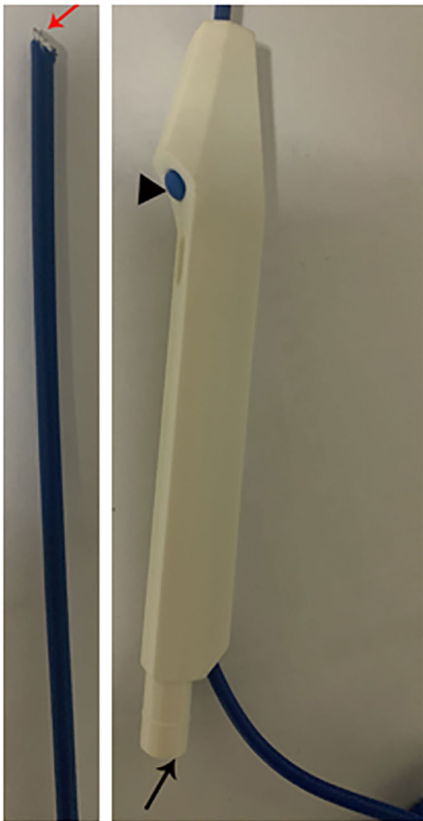
Fig. 1 Modified monopolar device. Red arrow indicated needle-like front-end, black arrow indicated a suction hole, black triangle indicated the button
