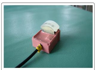
Figure 1 Used forced sensor for tension measurements developed by Applied Medical Engineering, Helmholtz Institute, RWTH Aachen, Germany.
