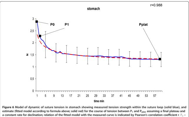
peak suture tension,  $P_1$  = transition to the constant declining phase,  $P_{plat}$  = suture tension of the constant plateau (mean ± SD).
