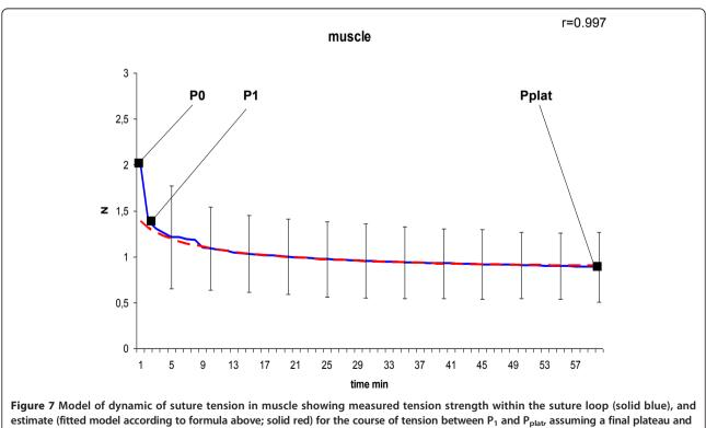
a constant rate for declination; relation of the fitted model with the measured curve is indicated by Pearson's correlation coefficient r.  $P_0 =$  peak suture tension,  $P_1 =$  transition to the constant declining phase,  $P_{plat} =$  suture tension of the constant plateau (mean  $\pm$  SD).
